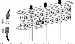
Replace 2x screws, 3x marble orbs and rods and brass plate to top of fixture, gently tightening against glass shade.
