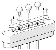
Disconnect electrical connectors and remove unwanted LED tape by carefully peeling off aluminium mounting block.
