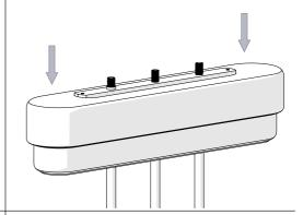
Replace brass plate, 2x screws and 3x marble orbs and rods to top of fixture, gently tightening against glass shade.
